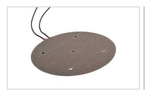
The mica heating element consists of a resistive element insulated between two layers of micanite. Mica heaters are of varied rigidity and have the capability to work at higher temperatures. These type of heaters need to be mechanically fixed onto the application in order to guarantee optimal heat transfer.
