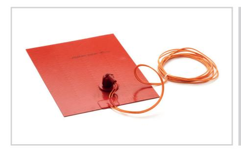
The silicone heater consists of an etched foil resistive element which is laminated between two layers of silicone rubber achieved by a vulcanizing process that delivers a high mechanical stability for the flexible and light weight heating element. As silicone is a robust material with excellent temperature proprieties, it can be used in both high and low temperature applications. Reinforced fiberglass-silicone rubber gives the heater dimensional stability without sacrificing flexibility.
